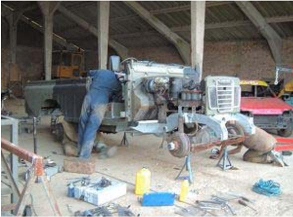
The rear body also took four people to lift on, but it seemed more manageable than the bulkhead. Woodworking clamps were needed to pull the body towards the chassis to make the bolt holes line up.
