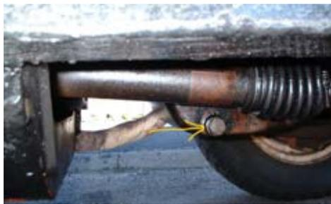
Be prepared for the sudden flow of oil as you remove it, as initially it will come out with some force. Leave the sump to drain whilst you concentrate on the oil filter, which is in a canister mounted on the driver's side of the engine:
