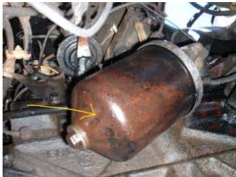
Undo the 5/8" bolt, and the canister will come loose – there are roughly 1.5 pints of oil in there, which will issue out of the higher part of the housing as you loosen it. It's situated in such a position that the oil will drop onto the front propshaft before reaching the oil catching container, so that might need repositioning to catch the oil. (Odds are, you will get a goodly amount running down your arm too!)
