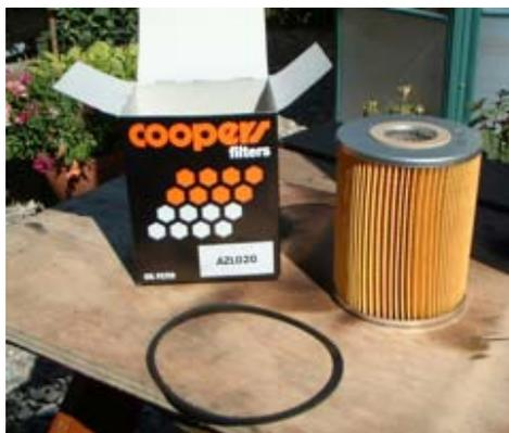
Fit the new seal, remembering to give it a smear of new oil first. Now refit the canister and filter. It might take a bit of jiggling to get the bolt back in the housing, so be prepared. Patience will win out!
