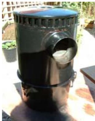
Keeping it the right way up, undo the three clasps holding the two sections of the canister together, and carefully remove the top section. There is a wire mesh section in the bottom part of the assembly; remove this and then drain the old oil out of the container:
