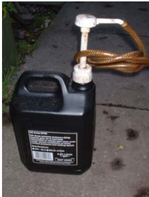
Once the gearbox is full, the oil will start to come back out of the filler aperture; now you can replace the filler plug. Remember, you can check the oil level in the gearbox at any time by removing this plug....just allow time for the oil to settle after a run....and top it up as necessary.
