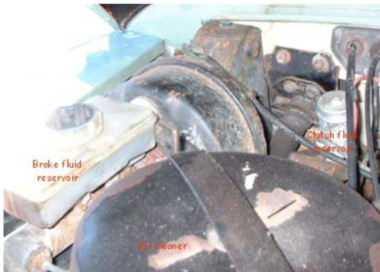
On later models these are separate, as in the photo (though there isn't always a brake servo fitted), but some earlier models have a metal can which contains the fluid for both systems. There is an inner and outer container, and there should ideally have a level amount of fluid in each.
