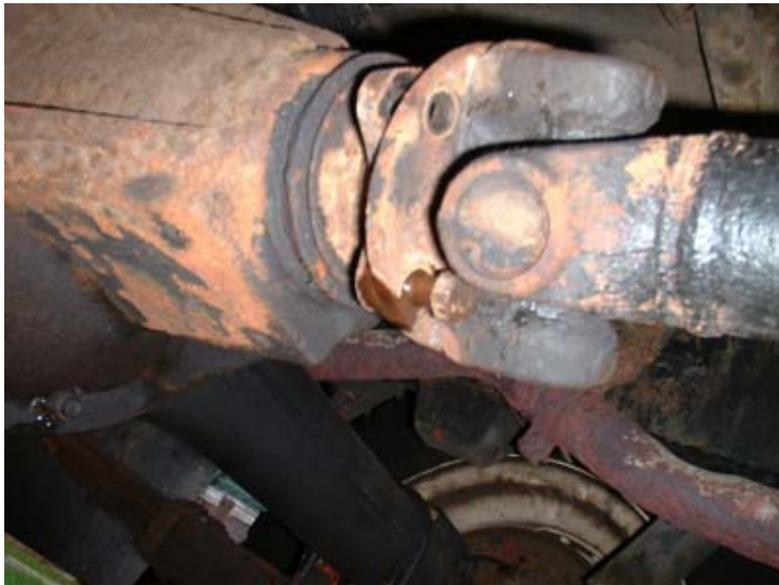
Remember to replace these bolts and nuts with new ones!! (Second-hand ones have a nasty tendency to come undone, with quite disastrous results which are unpleasant to say the least!) You won't need to undo the handbrake drum end, just support the propshaft out of the way by tying it to the crossmember above.
