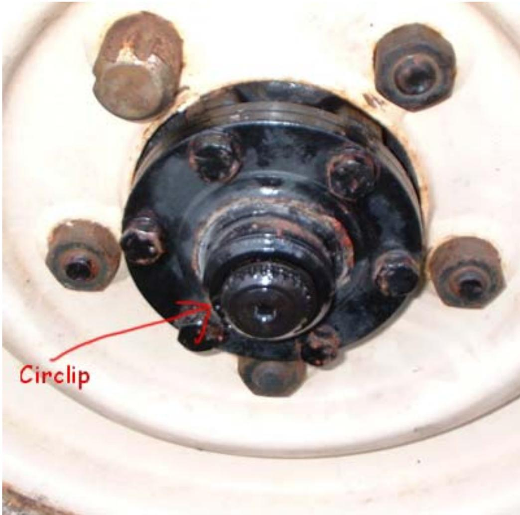
As you can see, the top hat has been removed and the drive flange is held on with a circlip. The next photo shows an earlier 10 spline half-shaft, with a split pin and castle nut:
