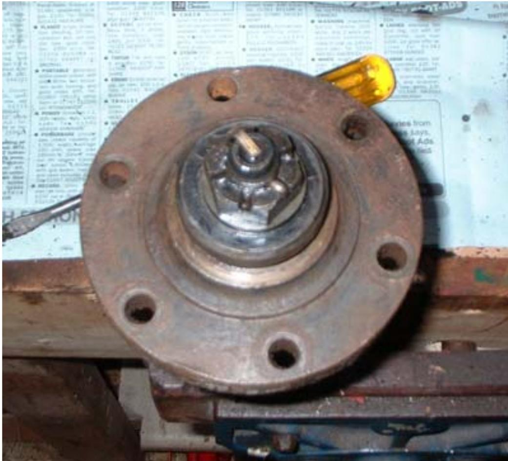
To find which shaft has broken, undo the 6 bolts holding the drive flange to the hub; no need to remove the wheel at this point:
