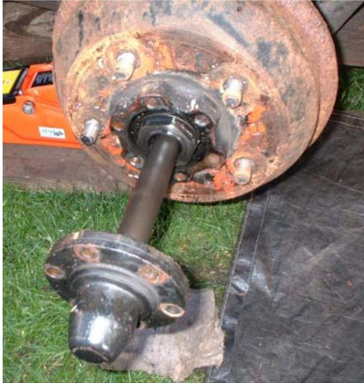
You will soon see which is broken!! In this instance it was the shorter shaft, on the driver's side:
