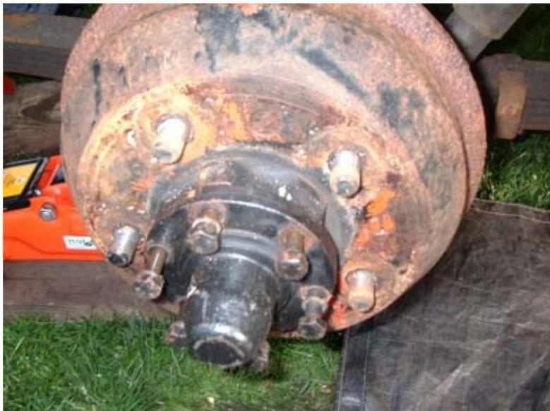
and then withdraw the half-shaft and drive flange complete:
