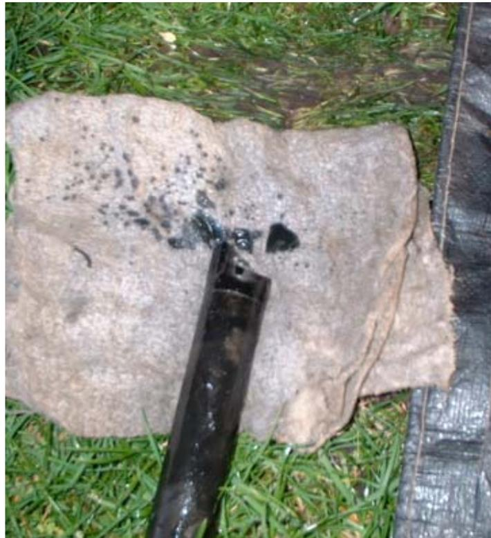
The longer shaft had evidence of wear on the splines when it was removed, so I decided to replace both shafts. They cost £13.90 each, so it made sense to do them both at the same time.
