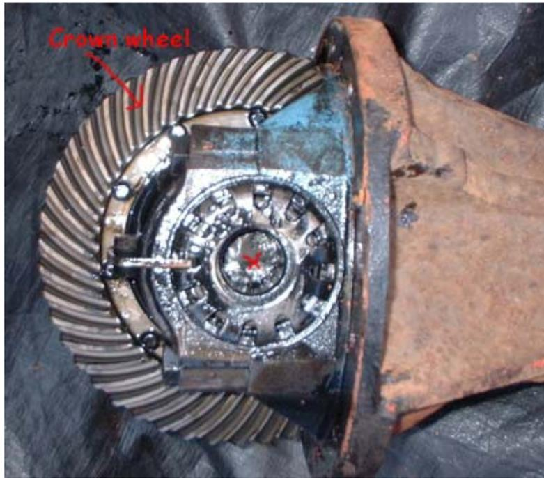
To remove the remaining piece of shaft, turn the diff over, and, from the other side, use a long thin chisel or screwdriver to tap the offending article out ... it might be a bit stubborn!
